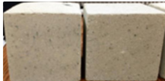
Figure 6: Samples with 90% Glass Sand.
