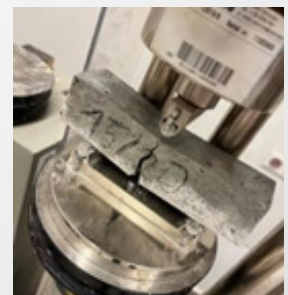
Figure 3. Bending strength test - sample with 15x20 content.
